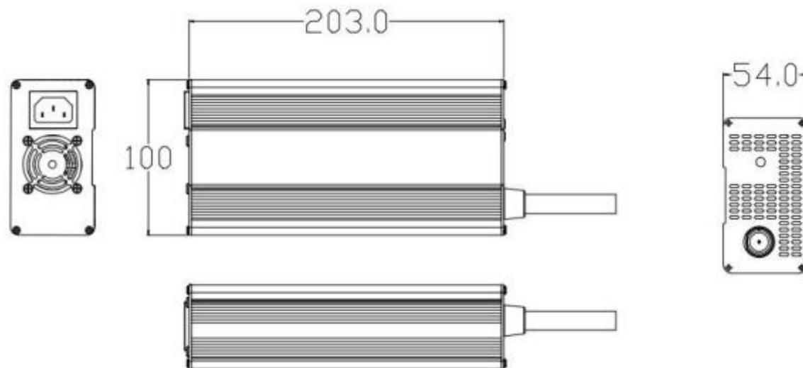
Tolerance of outline dimension is  $\pm 0.5$  mm , others are  $\pm 0.2$  mm in the diagram;
